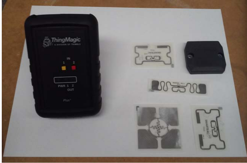
Fig. 3.1 RFID Reader and an assortment of RFID tags which were used
