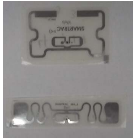
Fig 2.2 Flexible label Passive RFID tag
