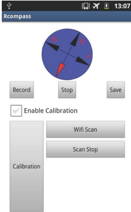
Fig 3.13a User Interface of Wi-Fi Compass. Program used to collect Wi-Fi data
